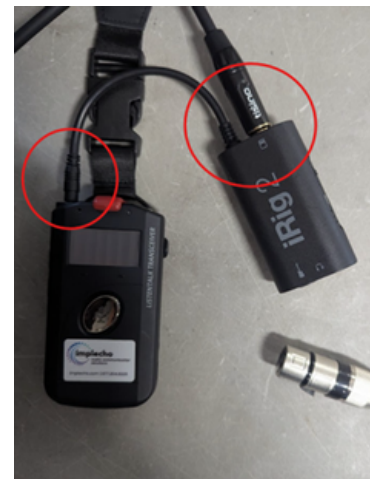
iRIG cable connection through a laptop connection on the soundboard
